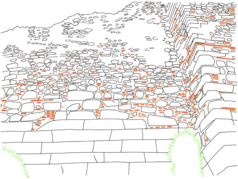
Fig. 93. Nea Kerassounda, Castle of Rogoi, tower 'IE'. View and drawing of a section of masonry.
